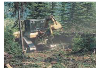
A crawler tractor or skidder with a grapple picks up bunched trees and drags them to a landing or roadside. Some grapples can swing 180 degrees, making it easier to operate in tight spaces.
