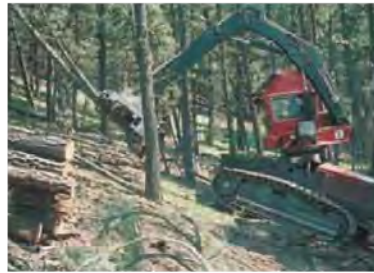
A feller-buncher severs trees and lays them in bunches with limbs and tops attached. Bunches are oriented with tree trunks facing downhill.
